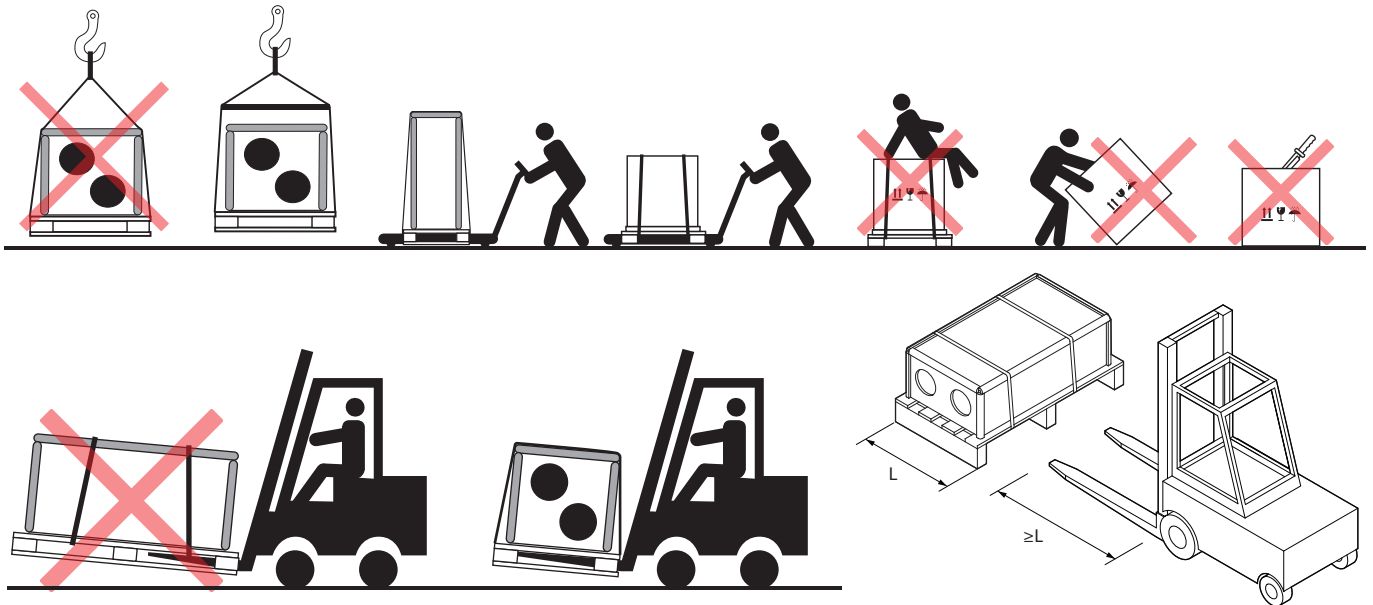
Fig. 4. Examples of transportation by crane, forklift and trolley
