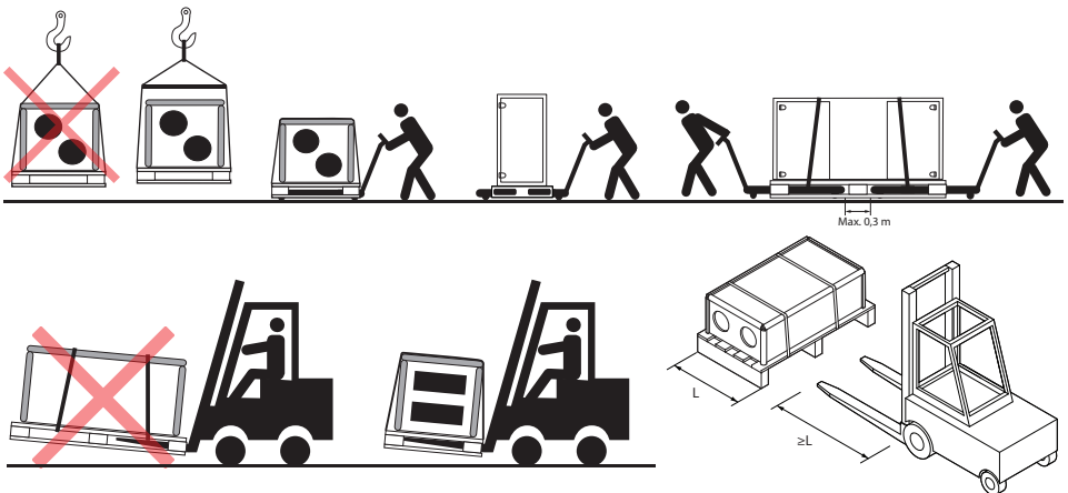
Fig. 5. Examples of transportation by crane, forklift and trolley
